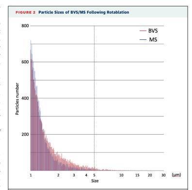
Absolute number of particles is indicated on the y-axis, and the semilog of particle size is indicated on the x-axis. It was found that 98.5% of bioresorbable vascular scaffold (BVS) particle and 99.3% of metallic stent (MS) particle were under 5  $\mu$ m in diameter.
