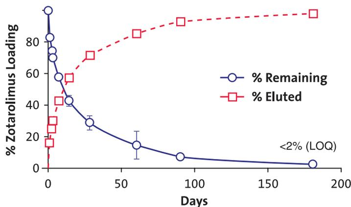
**Figure 2. The In Vivo Elution of the Resolute Zotarolimus-Eluting Stent System**
