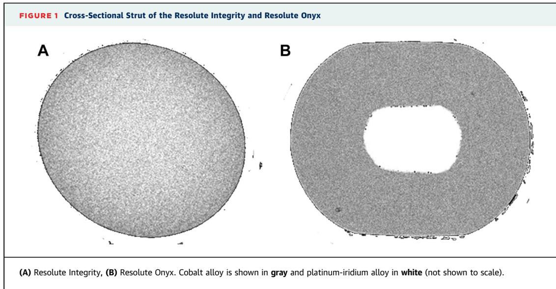
density of 8.4 g/cm<sup>3</sup>), and R-Onyx uses the same zotarolimus dose and polymer. However, R-Onyx has an inner core composed of a 90% platinum and 10% iridium alloy with a material density of 21.5 g/cm<sup>3</sup> (Figure 1). The higher density of the platinum-iridium alloy inner core used in R-Onyx
